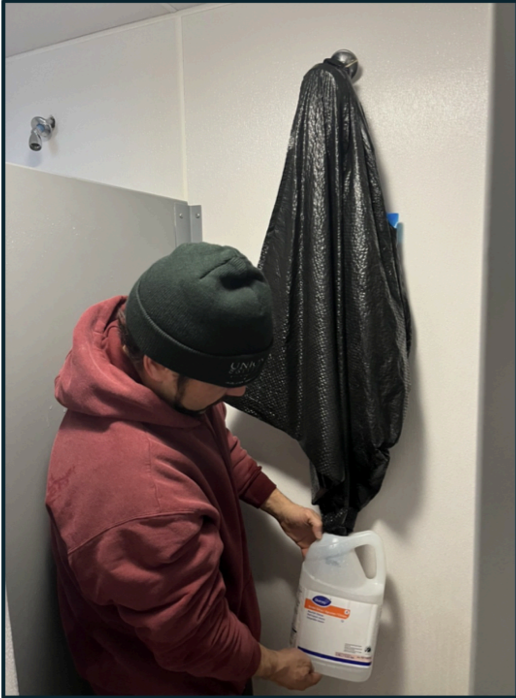
Image 1: Mark Moreau measuring the flow rate of a showerhead using the method described above in Raymond House, Union College.
